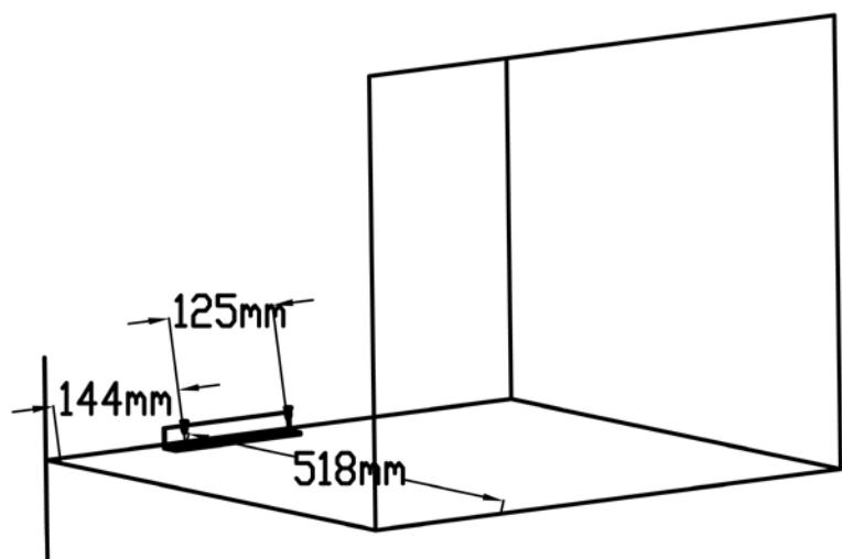
3. Before installing in a kitchen unit, screw the attachment plate provided onto the appliance with screws (4x15).
