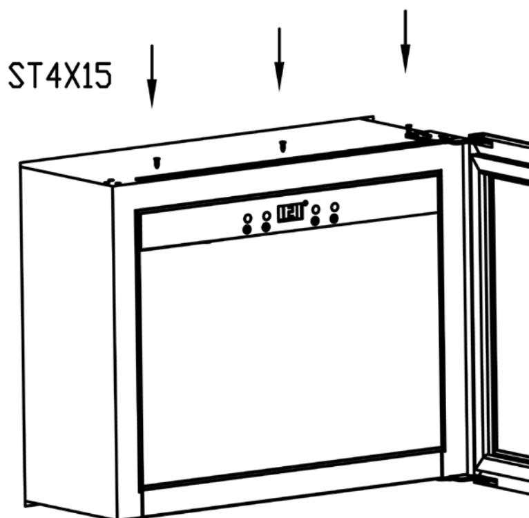
4. Slide the appliance into the recess leaving a 26 mm gap between the body of the unit and the front face of the door.
